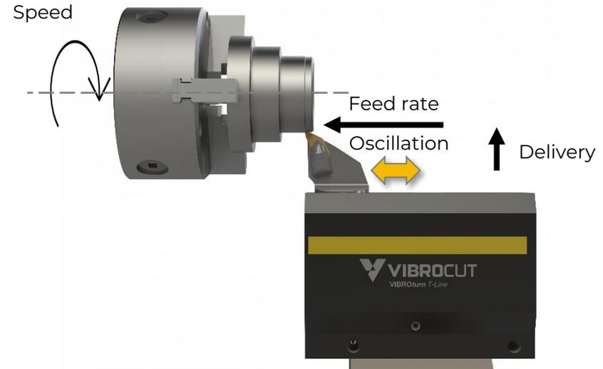
**Objective:** Realization of an economical and robust chip breaking behavior
