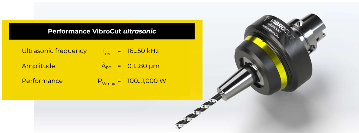
Figure 6: Ultrasonic tool holder VibroCut ultrasonic
