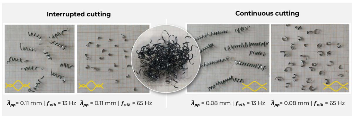
Figure 3: Influencing chip breaking with VibroCut oscillate (conventional chip shape - center)
