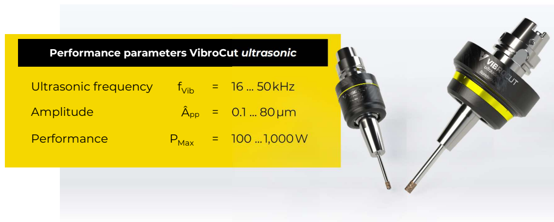
Figure 6: Ultrasonic tool holder for VibroCut ultrasonic
