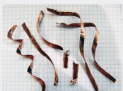
Ribbon chips and spiral chips
